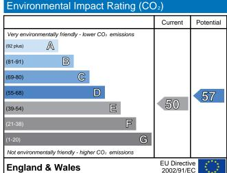
The environmental impact rating is a measure of a home's impact on the environment in terms of carbon dioxide (CO<sub>2</sub>) emissions. The higher the rating the less impact it has on the environment.
